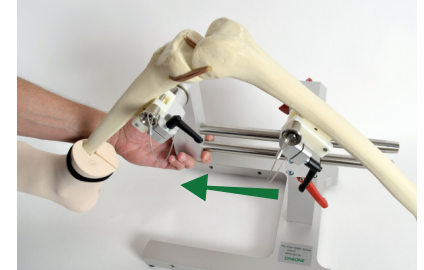
To set the leg in extension loosen all the red levers and pull on the guiding rail for the required extension
