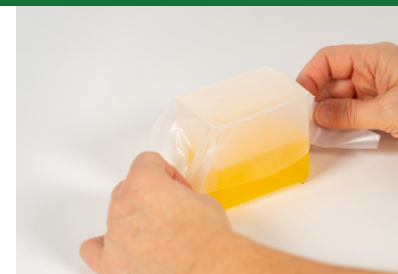
Place a small Parafilm cover over the entire opening and around the sides of the bladder container
