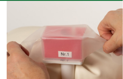
Pull down the Parafilm cover under the holder and ensure the entire opening is covered and sealed
