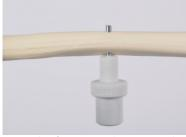
Insert the first DFO adapter into the hole of the femur bone model
