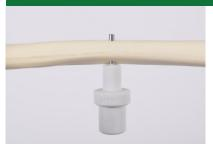
Insert the first DFO adapter into the hole of the femur bone model
