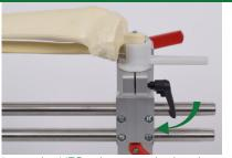
Insert the HTO adapter to the bracket of the supporting column and tighten the locking lever with slight pressure
