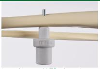
Insert the second HTO adapter into the hole of the tibia bone model
