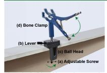
Place the ball head bone clamp on the table, tighten the screw firmly. Use the lever to lock/unlock the ball head.
