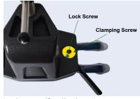
Lock screw (Small); clamping screw (Big)
