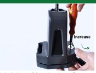
Unlock the ball by using lever. Remove the lock screw.
