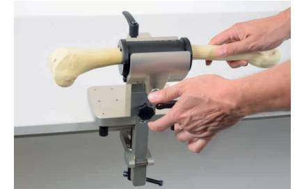
Place the SYNBONE® bone model into the Sleeve Clamp and tighten the locking lever with slight pressure
