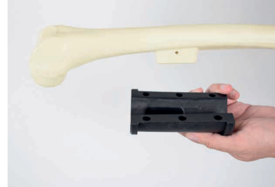
Insert the notch of the SYNBONE® femur model into the matching femur sleeve
