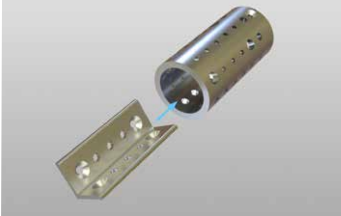
Insert the L-Profile into the Shaft Sleeve
