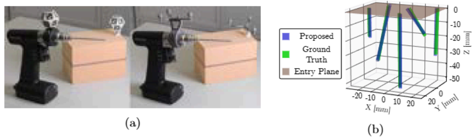
Fig. 5: (a) Mock surgical procedure with a drill and foam block and (b) digital twin of the drill holes from the proposed system compared to the ground truth.
