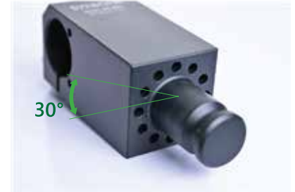
The Base Adapter's circular hole arrangement allows mounting positions in 30° steps. Page 3 for more details.
